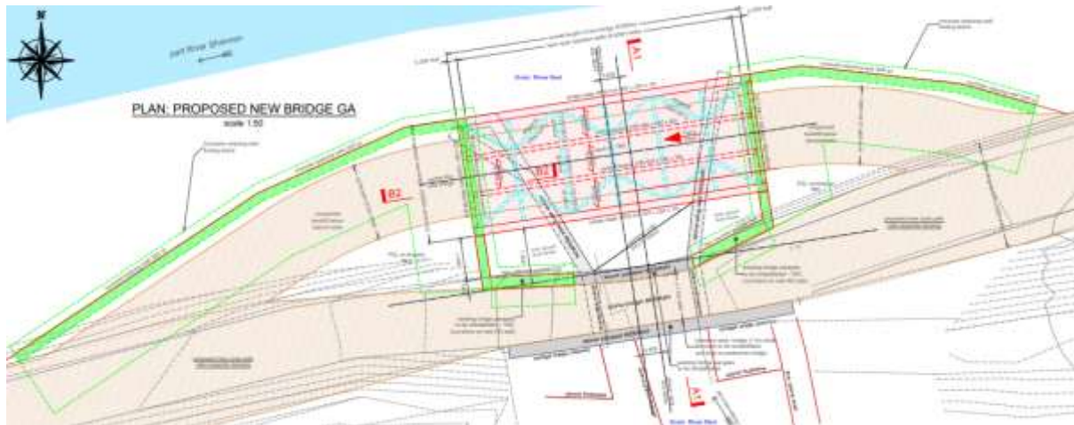
Figure 6-90: Plan for the proposed new bridge 2 alongside the existing stone bridge (refer to drawing RHA-XX-DR-S-SP0021)
