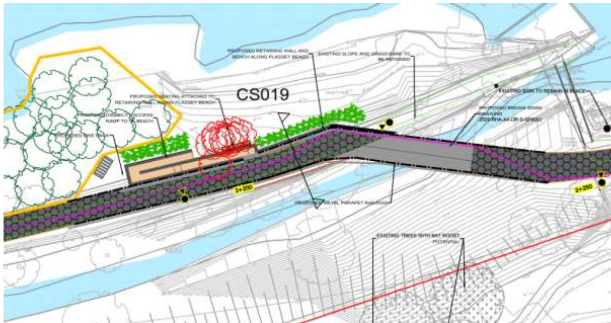
Figure 6-105: Proposed plan of ramp and Bridge 5 at Plassey Beach
